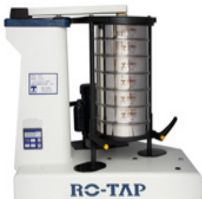
Figure 1. Tyler Ro-tap Shaker Machine with Sieve Stack
