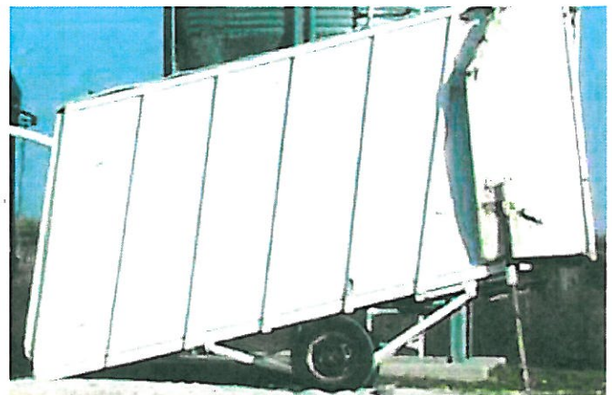
Fig. 1: Traditional metal covered chute (T). The chute was 76.2 cm in width, 2.3 m in height, and 4.6 m in length, and used square stock (2.5 cm) metal cleats which were spaced 20.3 cm apart.
