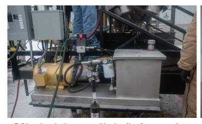
7.5 hp electrical motor and hydraulics for v-restrainer
