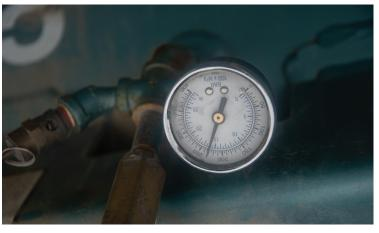
Presssure gauge on air compressor tank
