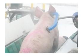
**WARNING:** The stunner wand operator must be sure that the foot pedal depressed and wand button pressed only after the wand is securely held into place on the pig. The button should be released as soon as the desired contact time is reached. The stunner wand operator must be sure that the wand does not make contact with any metal surfaces while the button is pressed.
