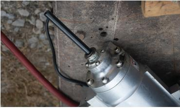
Extended bolt from the pneumatic captive bolt gun
