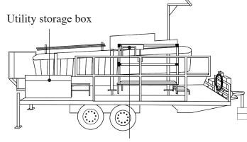
The electrical stunner box placement location is on the elevated stand.
